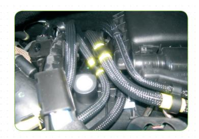
Easily installed thanks to its expanding diameter capacity (approximately 1 to 2) enabling significant differences in cross sections, elbows, connections, etc to be overcome without kinks or flattening.
